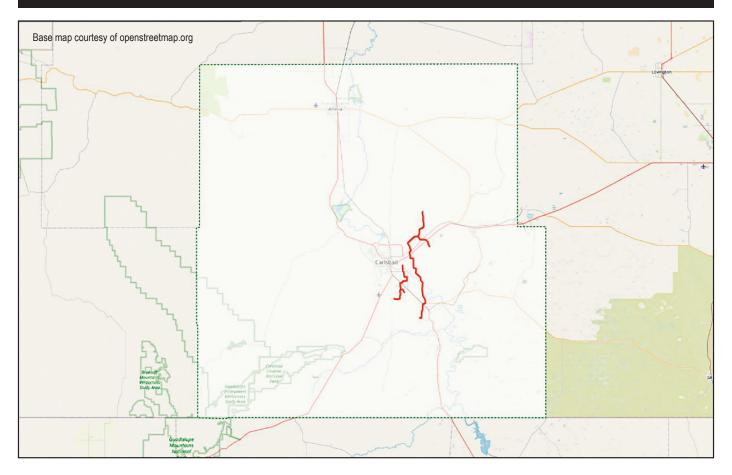
Trace Touchdown High Pressure Pipeline system is comprised of approximately 26 miles of 20" natural gas gathering lines and operates at 1480#.
